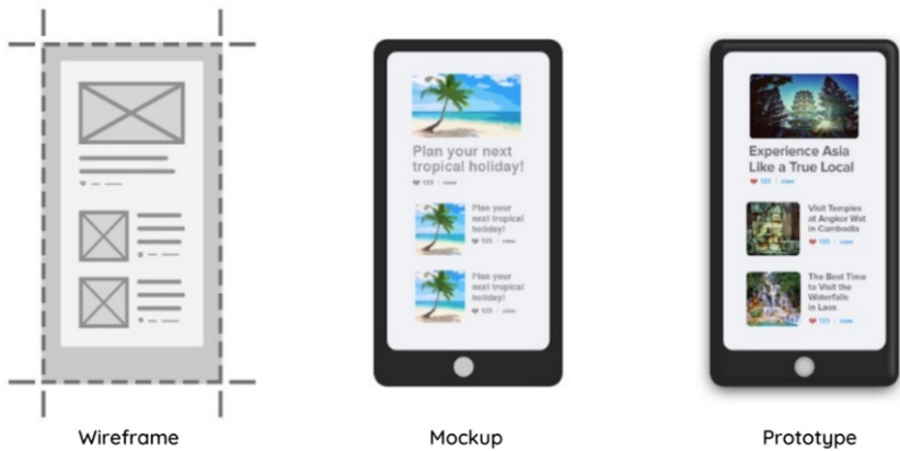
Figure 2: Wireframe, Mockup, and Prototype for the Travelling Platform (Example) 2
